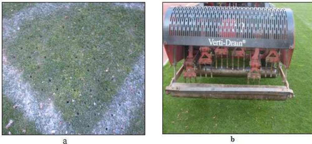
Figure 1: Soil mechanical aeration, a: perforated turf, b: turf aerator
